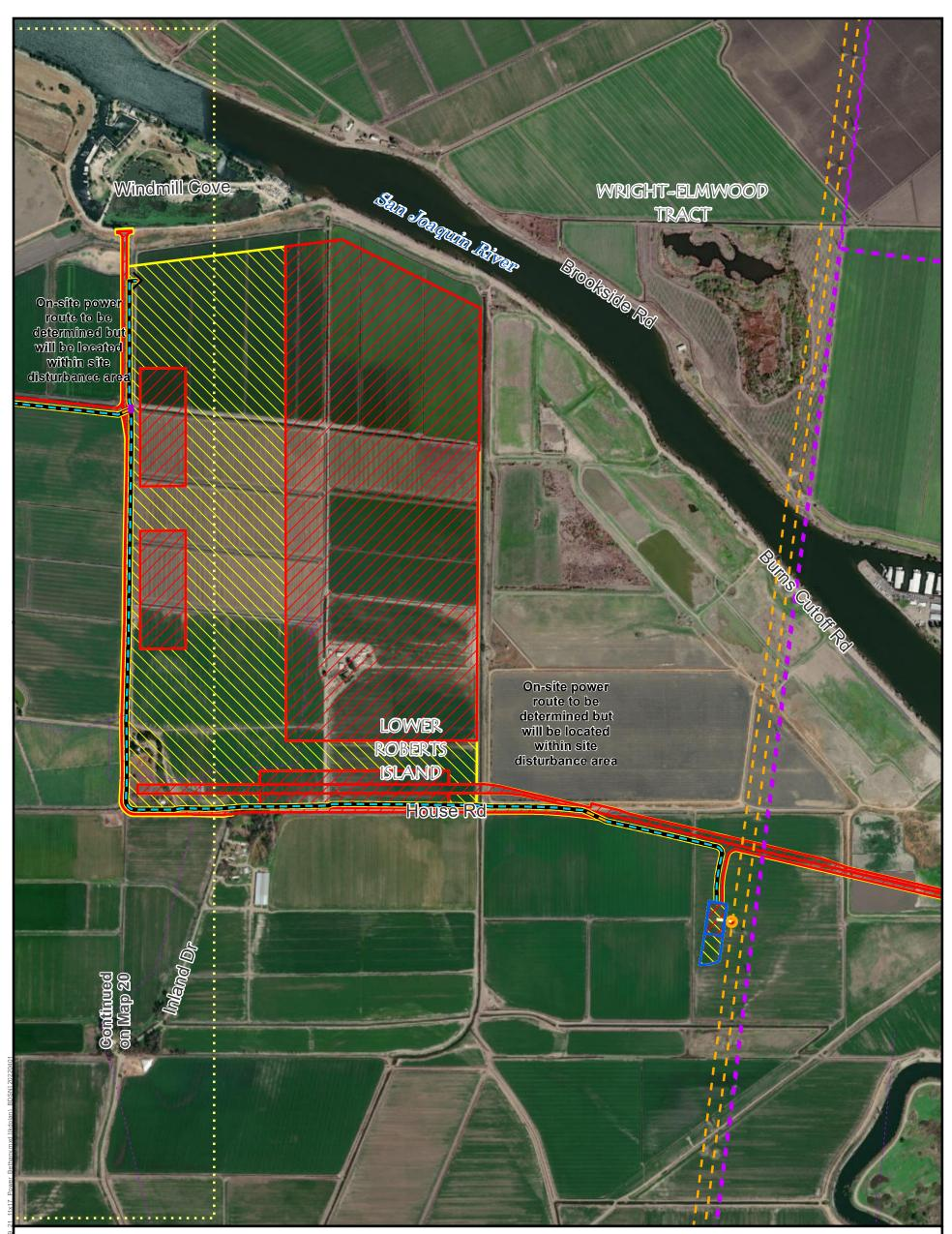
Page Index Connection to Existing Overhead Proposed Substation Proposed Switching Station Proposed Underground Power Within Proposed Roadway Outside Roadway Proposed Overhead Power New Line and Poles Existing Power PG&E Low Voltage ----- 11 kV PG&E High Voltage ----- 230 kV WAPA ------ 230 kV Permanent Subsurface Impact Permanent Surface Impact Temporary Surface Impact
