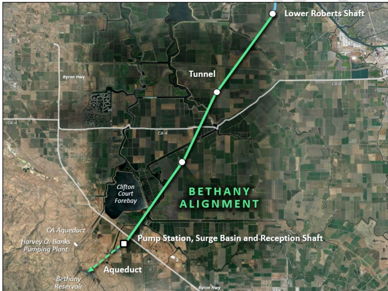
Figure 1. Delta Conveyance Project, Bethany Reservoir Alternative Schematic, South of Lower Roberts Shaft
