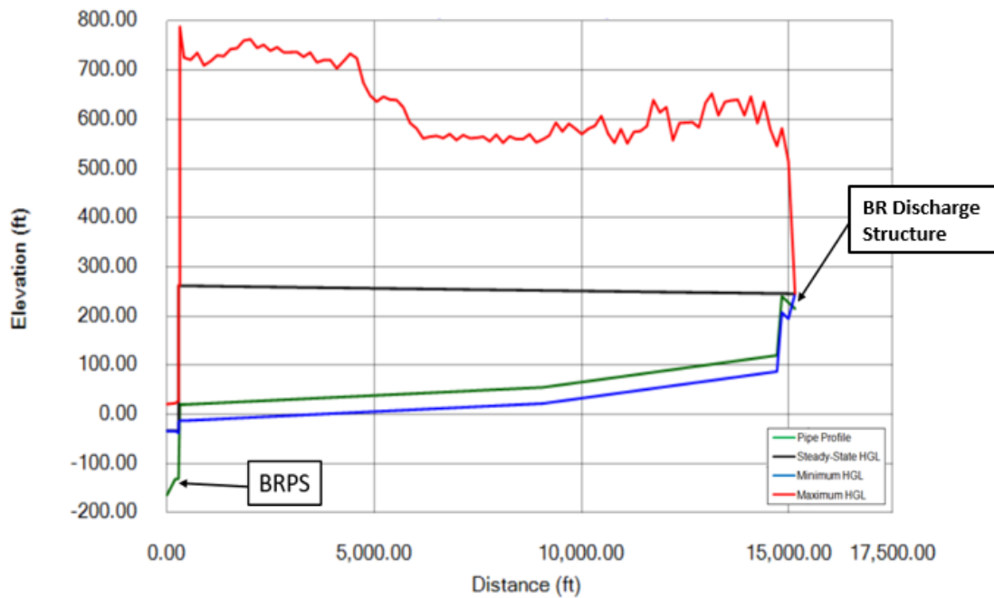
Figure 1. Surge Mitigation Alternative 1 - No Surge Mitigation Facilities for Bethany Reservoir Aqueduct Pipelines: Maximum and Minimum Hydraulic Gradeline Profiles
