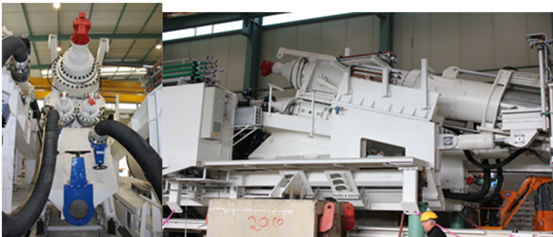
Fig. 3: Slurryfier-box with stone crusher for 7m diameter TBM (Kuala Lumpur)
